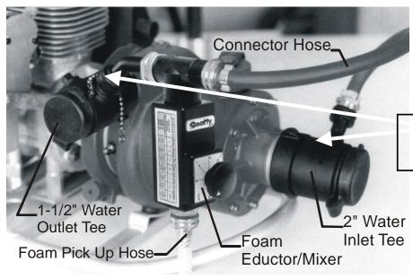
4. Start pump and water flow. Control foam induction by opening the Foam Control Knob Inductor/Mixer to desired foam percentage. (See percentage induction guide label on side of unit).
