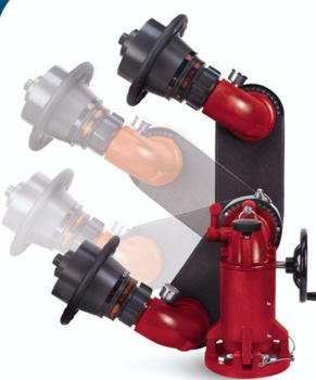
The Apollo Hi-Riser, includes the outstanding features of the standard Apollo along with the added benefit of rising over obstacles on top of the fire truck. No inefficient extension devices or cumbersome telescoping pipes. Simply pull a pin and raise the discharge to a full 24" above the base. Also, the Apollo Hi-Riser rotates easily down to a low profile position for portable operation and comes complete with an automatic drain valve.
