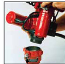
2" Quick-Disconnect, Ideal for Cab Forward Trucks
