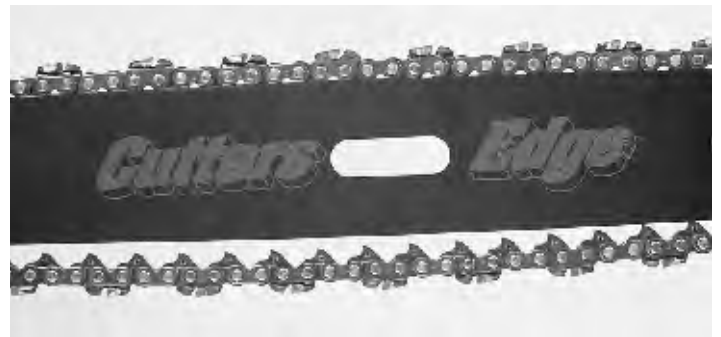
Fig. 9 "Sag" chain is too loose
