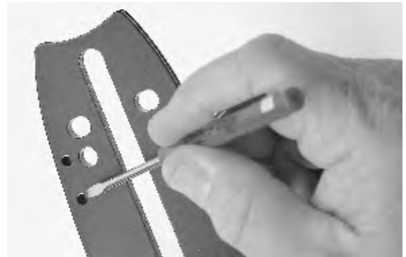
Fig. 28. Cleaning oil holes on guide bar
