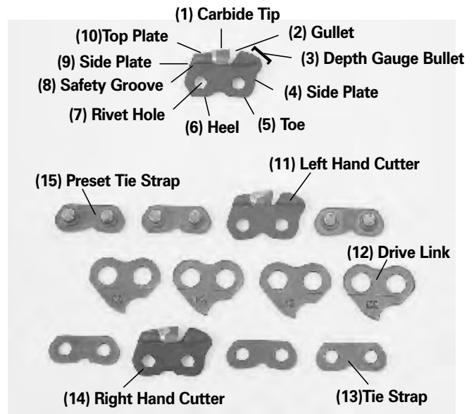
Fig. 26. Components of the BULLET® CHAIN
