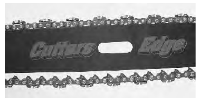
Fig. 16 The chain will sag when hot
