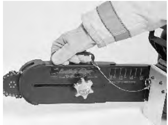
Fig. 21. Set to the desired depth of cut.
