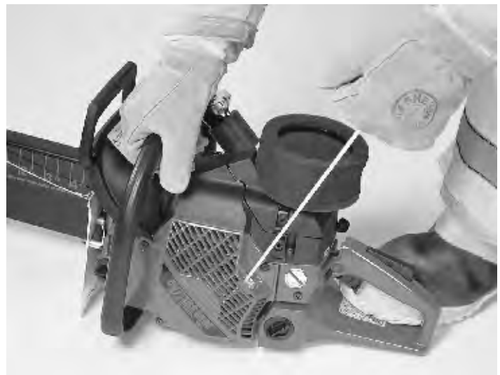
Fig. 13. Proper starting position
