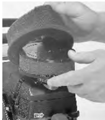
Fig. 33. Remove the Pre-filter
