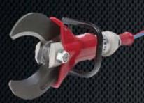
BRC-39/150 Medium Rescue Cutter is ideal for cutting most common materials found in road rescue, building collapse and earthquake disasters. Its powerful parrot beak jaws produce 39 tons of cutting force with a 150mm opening.
