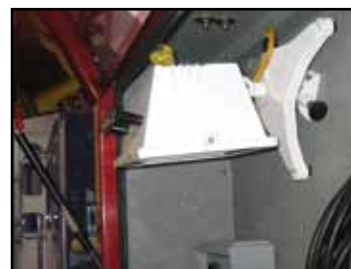
PLMT - can mount a PL Light on its side or upside down
