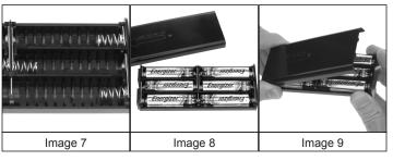
batteries are of one or the other model...do not use a combination of the two), install the batteries per the diagram located on the inside base of the battery carrier. (Image 7)
