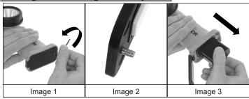
WARNING: To prevent ignition of a hazardous atmosphere, do not open the battery compartment in the hazardous environment. This task must ONLY be done in an area known to be non-hazardous.
