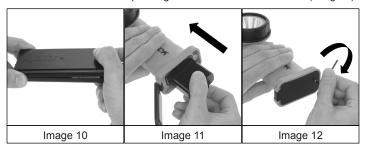
• While keeping the left-hand tabs in their slots, gently press down on the right side of the cover until the two right-hand tabs slip into their respective slots. (Image 10)
