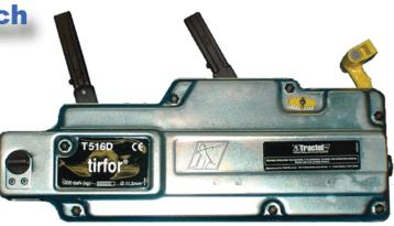
Hand Operated Tirfor machines are level operated hoists using a separate wire rope. Single-person operated, using a telescopic operating handle, they can work in any position and over any height of lifts. This winch can replace conventional winches and other hoists for many applications.
